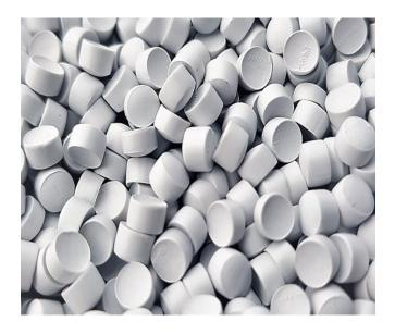
PVC Filler granule is the raw material for the production of the middle layer (the layer between the insulation and the sheathing) of the cable. Fillers are at a lower level than other polymer layers in terms of physical, mechanical and thermal stability properties and are used only to smooth the substrates and prepare the cable for sheathing.
