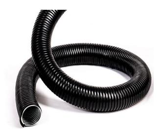
Flexible GI Conduit is used to protect wires and cables in construction. It is made of aluminum with a thin layer of PVC as a cover on its surface. Important features of this thin layer include high flexibility, good tensile strength, glossiness and polished surface of final product. Due to the fact that the main use of these flexible pipes is in the open space, it must have high resistance to UV rays, so they are mainly produced in white and black colors.
