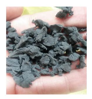
PVC flakes are produced from the waste of PVC cables, hoses, etc., and that product is usually used to produce shoe soles and hoses.
