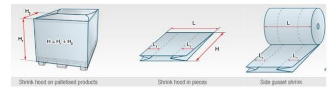
In order to increase the film's resistance to UV rays and also improve the shrinkage of the films, they are produced in multi-layers (co-extrusion).
